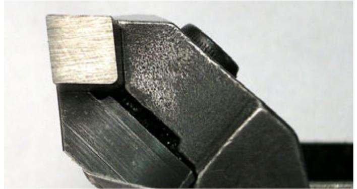
The tool bit can be ground on both ends. A radius point could be ground on one end and a sharp corner on the other. Just turn the bit over for a different profile.
